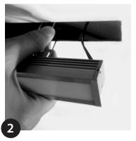
Slide spring clips to ensure even spacing. Secure with grub screws if desired. Compress spring clips, insert into slot and push flush.
